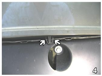
In the middle under the fascia, remove the two clips by pushing the sides of the clip together with a small screw driver. Set the clips aside to be reinstalled later.
