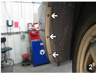
Just forward of the front tire, inside the wheel well, remove three bolts with a 7MM socket.
