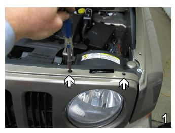
Remove seven bolts with a T20 Torx from across the top of the fascia (driver's side shown in photo). Set bolts aside to be reinstalled later.
